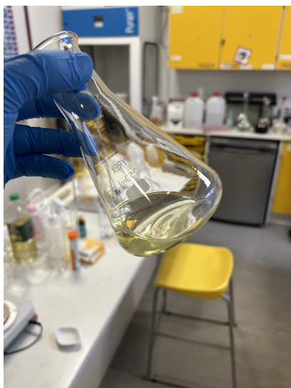
(a) H&B tablets in acidic solution (off-white before titration).
